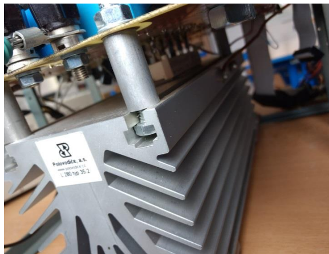
Figure 5.8 – Cooling Fin for Heat dissipation
