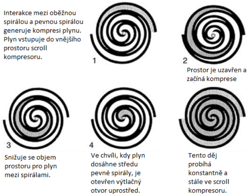
Obr. 19: Scroll kompresor a princip činnosti (Emerson Climate Technologies) [4]
