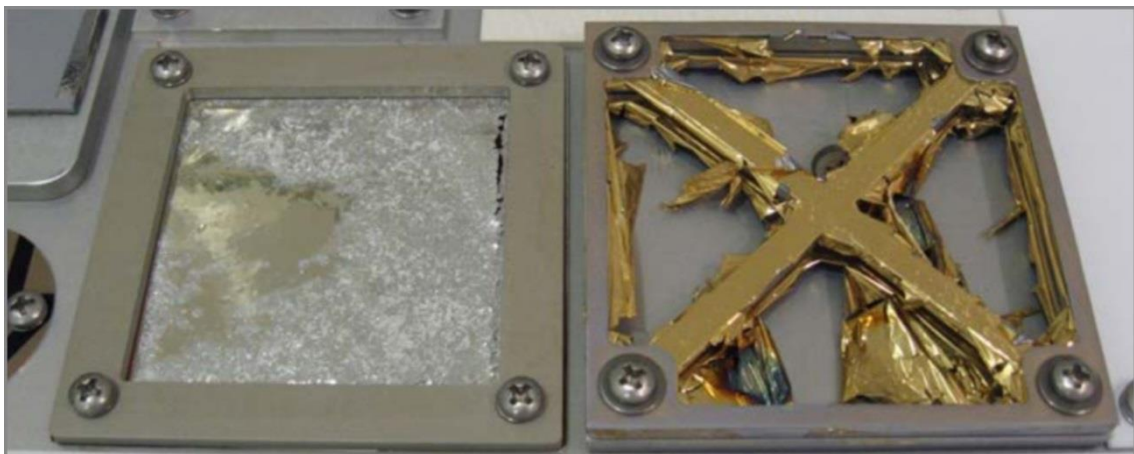
Figure 31: Outcomes of the ISS Material experiment 4 illustrating the failure of the coating resulting from the combination of thermal cycling and the exposure to atomic oxygen. [40]
