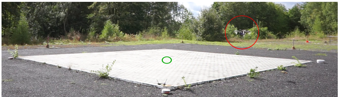
Figure 31 An outdoor area where the real experiments were conducted. The UAV is highlighted by a red circle. The concrete surface is a square of 10 \text{ m} \times 10 \text{ m} . The radiation source was placed in the center of the area marked by a green circle.
