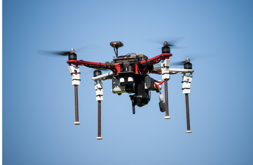
Figure 2 DJI FlameWheel F450, a medium-sized quadrotor and the primary target platform for the work presented in this thesis.
