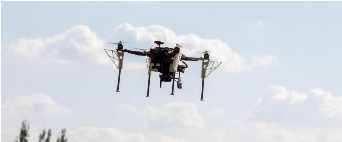
Figure 32 DJI FlameWheel F450 of the Multi-Robot Systems group. This quadrotor was used to carry the Timepix detector during the real experiments.
