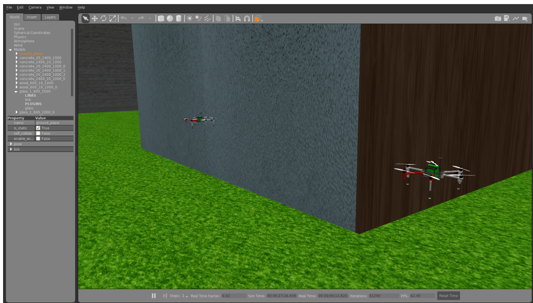
Figure 8 A screenshot from Gazebo showing the default graphical user interface (GUI) with a two F550 helicopters and a few obstacles with various textures. The UAVs bear a bright green marker. This indicates, that a UAV is carrying a Timepix sensor.
