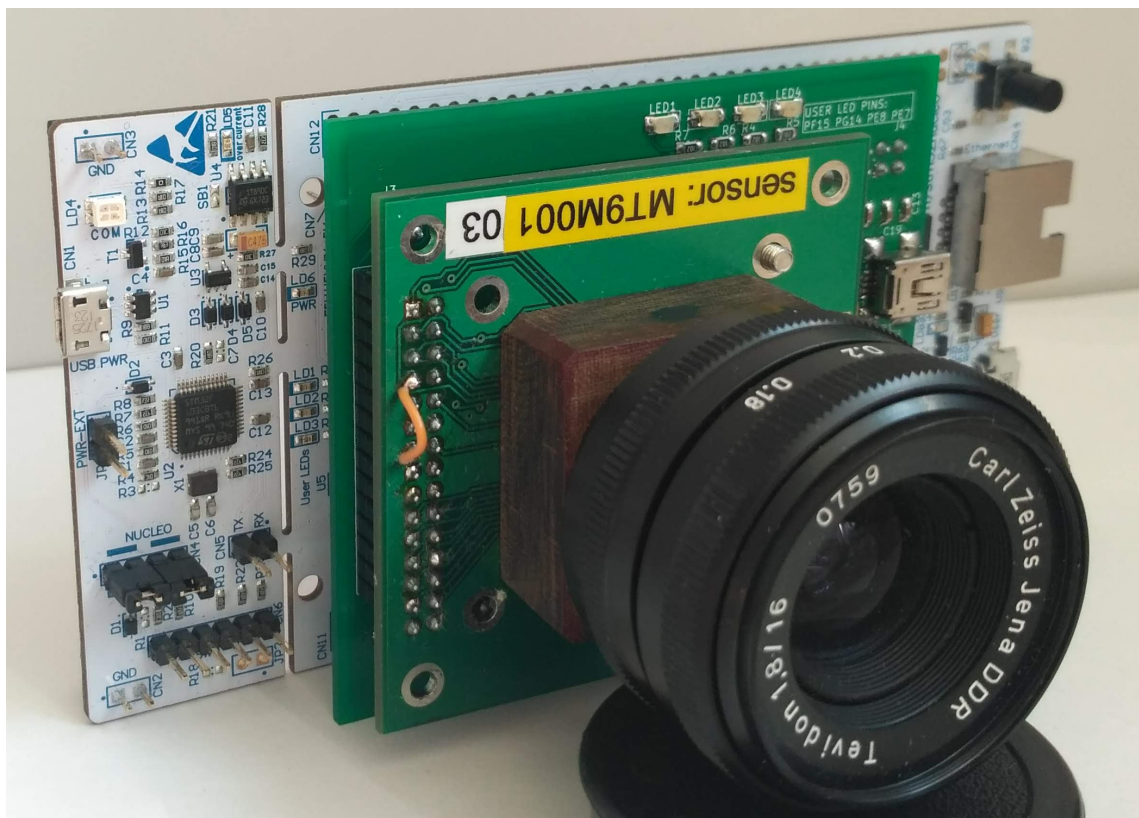
Figure C.9. Whole camera with final interfacing board
