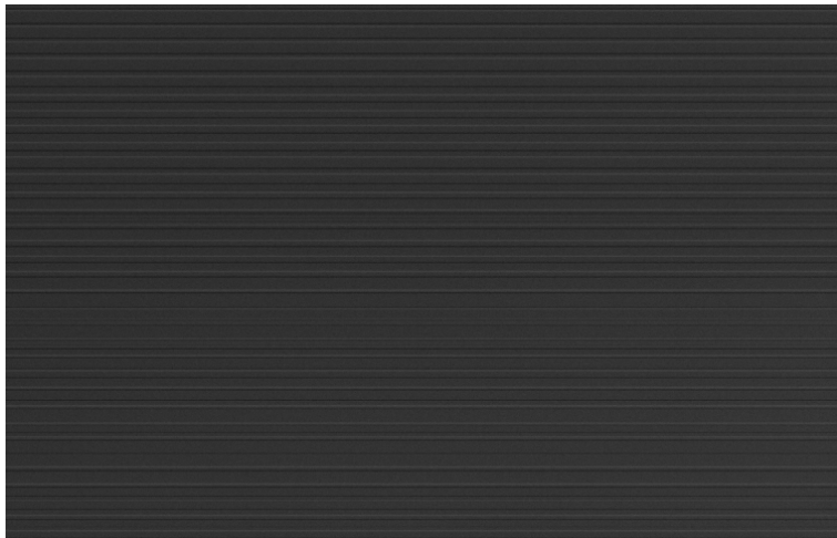
Figure 3.2. Image acquired from the camera: artifacts showing with higher px clock using the prototype of interfacing board
