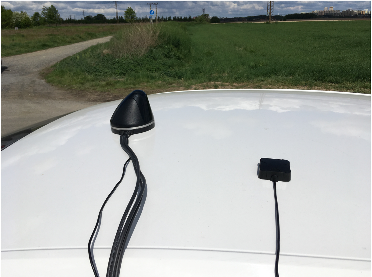
Figure 13: Antenna and GPS locator on the roof of the vehicle.
