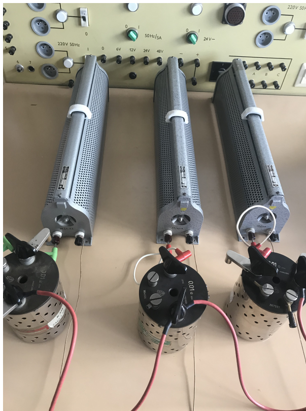
Figure 4.5: Rheostats and the reference 0.01 \Omega resistors
