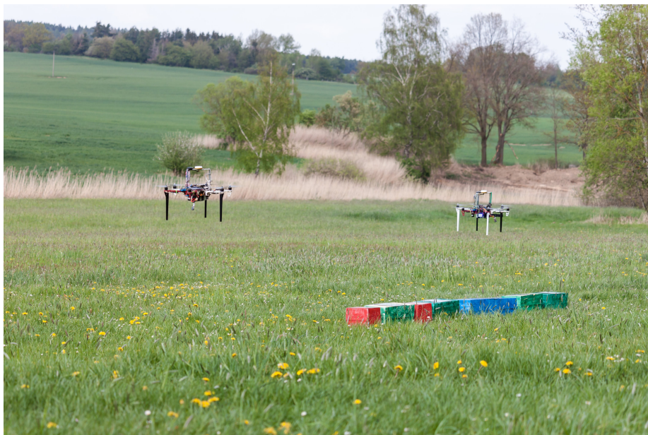
Figure 5.9: The UAVs in the waiting positions in front of the wall. The UAV that will enter the wall zone first is carrying the object of the color defined by planner to be placed as the next one in the wall.
