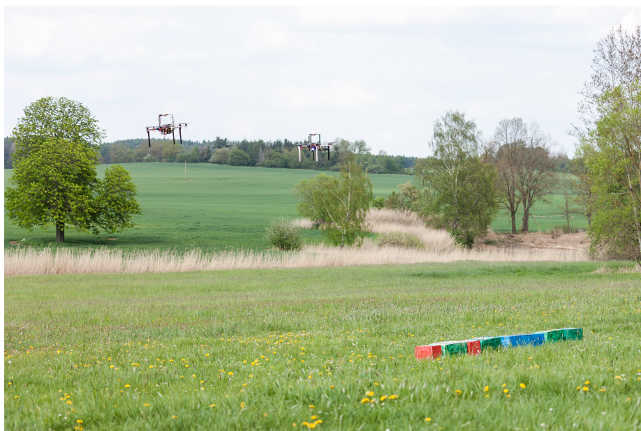
Figure 5.7: The UAVs flying to get brick shaped objects.
