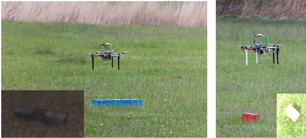
Figure 5.8: The UAVs attempting to grasp the blue and red colored bricks. On the corners of images, the views from the cameras on UAVs can be seen.
