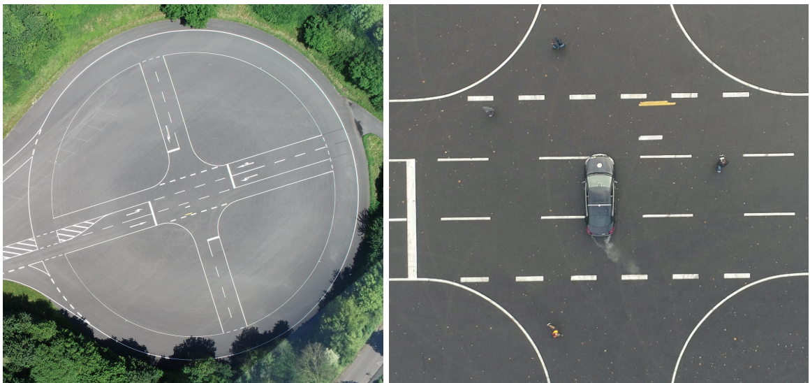
Fig. 4-5: Image of the measurement setup on the test track of the institute for automotive engineering. Four objects of the class pedestrian are visible. As no other objects exist around the test vehicle, all points recorded either belong to the ground or to a pedestrian.
