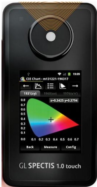
Fig. 33 GL SPECTIS 1.0 touch spectrometer [41]
