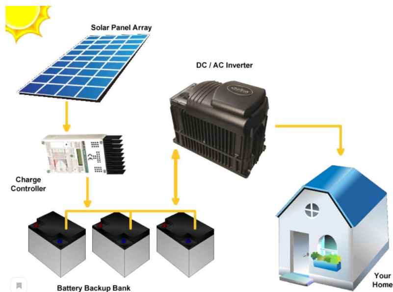
Figure 3 – Connection diagram of the PV system [12]
