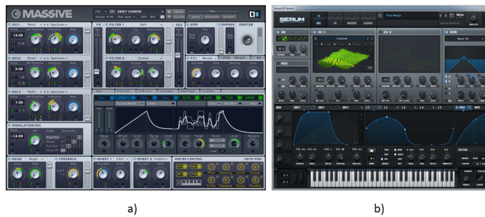
Figure 2.8: Popular VST-plugins for wavetable synthesis: a) – Massive, b) – Serum
