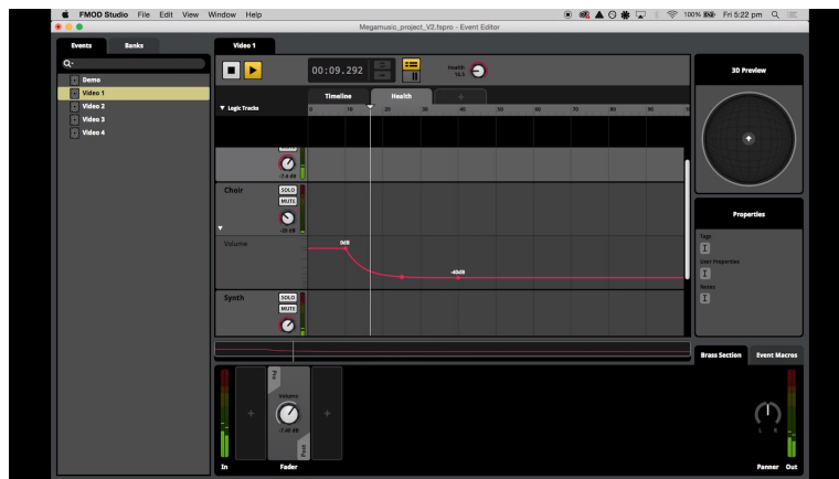
Figure 2.3: Example of volume automation within FMOD Studio. The curve drawn defines the volume that the "Choir" track will be played on depending of the value of parameter "Health".
