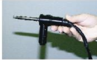
Figure 2: First generation of hand-held vital microscope with the principle of orthogonally polarized spectral imaging, taken from [64].
