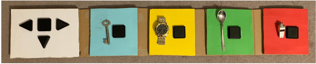
Figure 4.7: Design C: low-fidelity prototype of the OT divided into 5 sections, spatial orientation, navigation back to safety, time-related information, food related information and call for help
