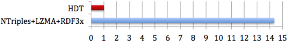
Figure 15: Comparison of HDT against with traditional techniques regarding the time to download and start querying a dataset [3]
