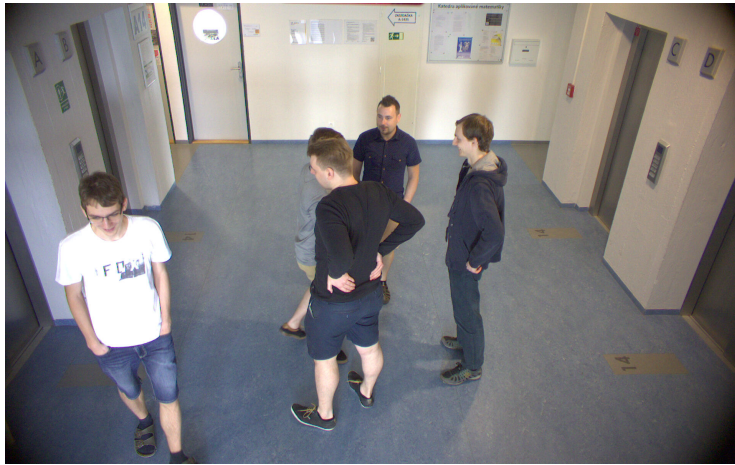
Figure 3.2: Example of the acquired image and the scene layout. We can see that despite being a quality lens, it contains distortion and vignetting.
