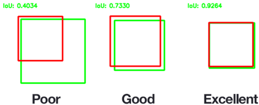
Figure 1.15: An example of computing Intersection over Unions for various bounding boxes. The predicted bounding boxes are drawn in red color, while the ground-truth ones are drawn in green color. Source: [14].
