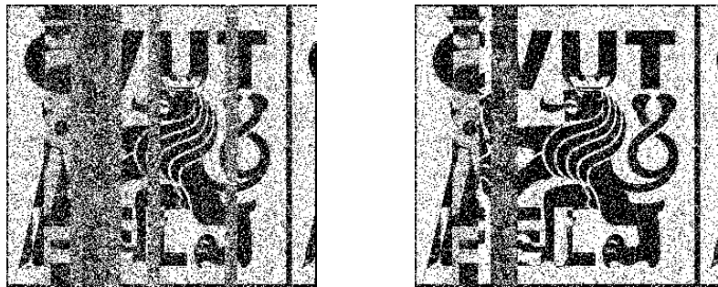
Figure 4.7. An example of received pictures resulted from the Butterfly network simulation run. There in a received picture in destination A,B from the relay, on the left. On the right, there is a received picture in relay from sources A and B in HMAC stage.
