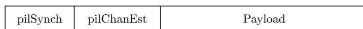
Figure 2.3. A frame composition for the transmission of source S_A and S_B in Phase 2 and Phase 3 of H-MAC stage.
