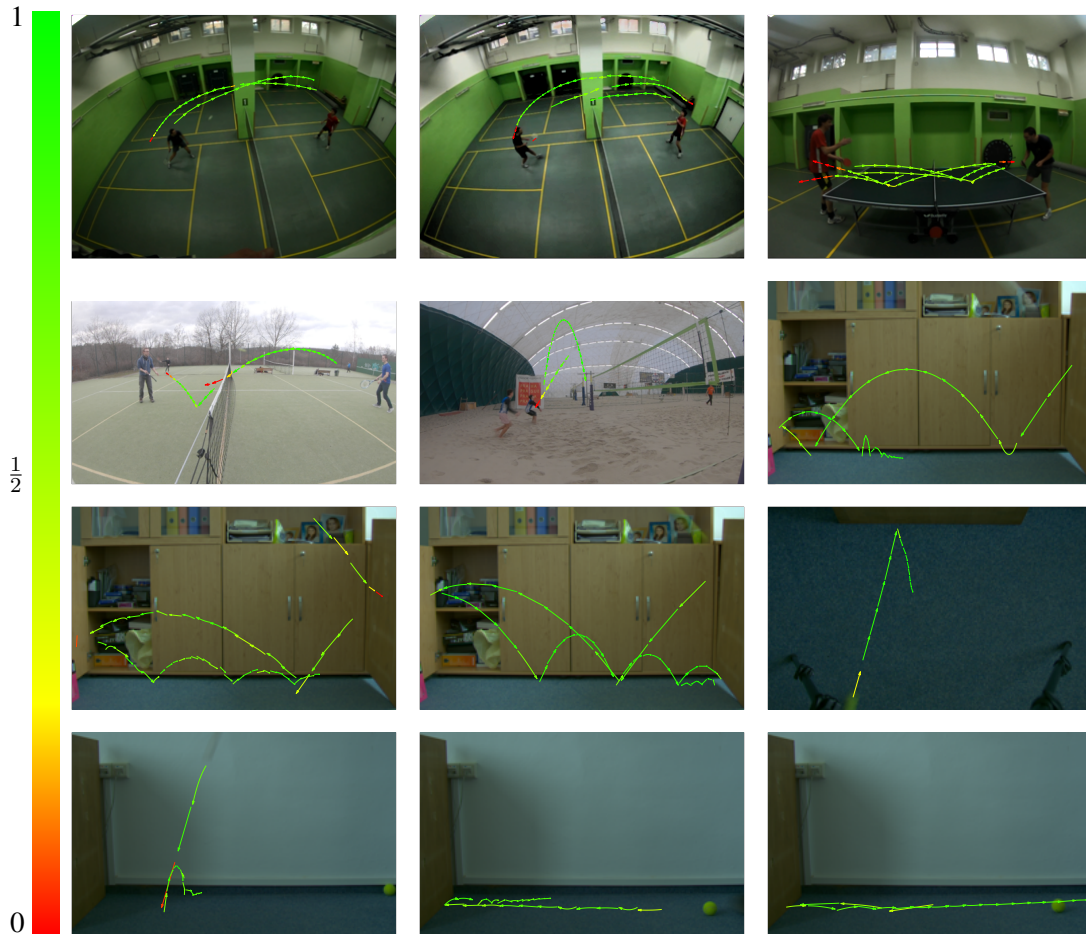
Figure 4.3. Trajectory recovery for all sequences from the TbD dataset. Trajectory Intersection over Union (TIoU (5.1)) with ground truth trajectories from a high-speed camera is colour coded by the scale on the left. Arrows indicate the direction of motion.
