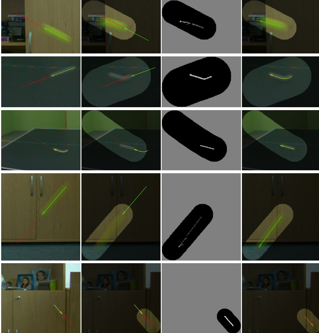
Figure 3.8. Examples of predictions in the TbD framework. From left to right: previous frame with estimated trajectory, current frame with predicted trajectory, estimated blur kernels, final trajectory fit in one frame. Predicted area in which computations are done is highlighted. Predictions are coloured in red. Current estimation of the trajectory is marked in a range from yellow to green, depending on the Trajectory-IoU.
