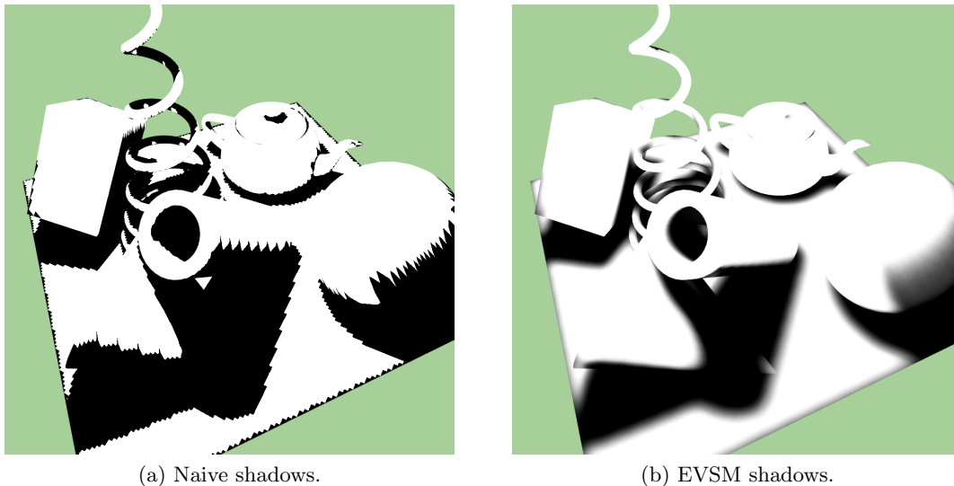
Figure B.2: Comparison of naive shadow mapping technique and EVSM with optimized 9x9 gaussian blur. Resolution of 256x256 depth map resolution.
