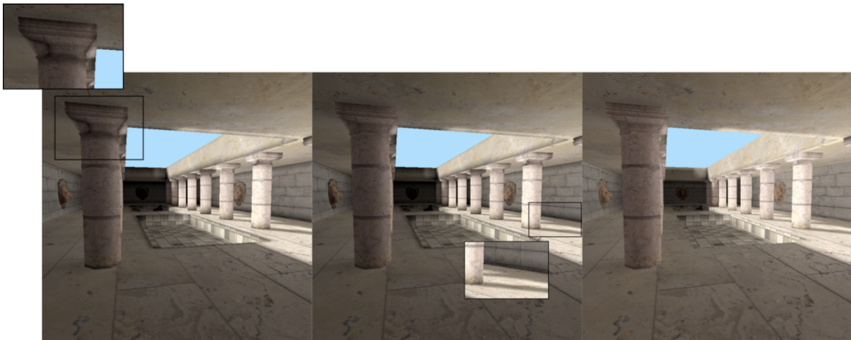
Figure 5.33. Pixel border extension, from the left to the right: No border extension, border extension only in LOD 0, border extension in all LODs. Wrong color blending is highlighted.
