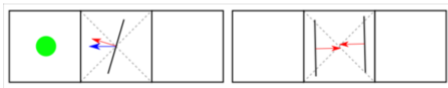
Figure 3.13. Voxel normal consistency check. On the left: the red arrow is a normal vector of the object, the blue arrow is a normal vector of the voxel. On the right: no normal vector of the voxel.
