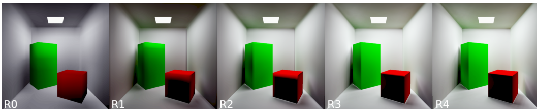
Figure 5.6. Testing renders for a different number of receivers, from the left to the right, from the lowest to the highest.
