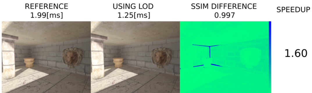
Figure 5.32. Camera View Dependant Zones in LOD. On the left: NO camera view dependant zones, 229 076 computed receivers. In the middle: WITH camera view dependant zones, 105 259 computed receivers. On the right is the SSIM comparison. A complete number of receivers is 335 015.
