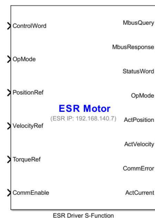
Figure 2.1: Simulink® block using S-function for MicroLabBox/ESR driver Modbus communication
