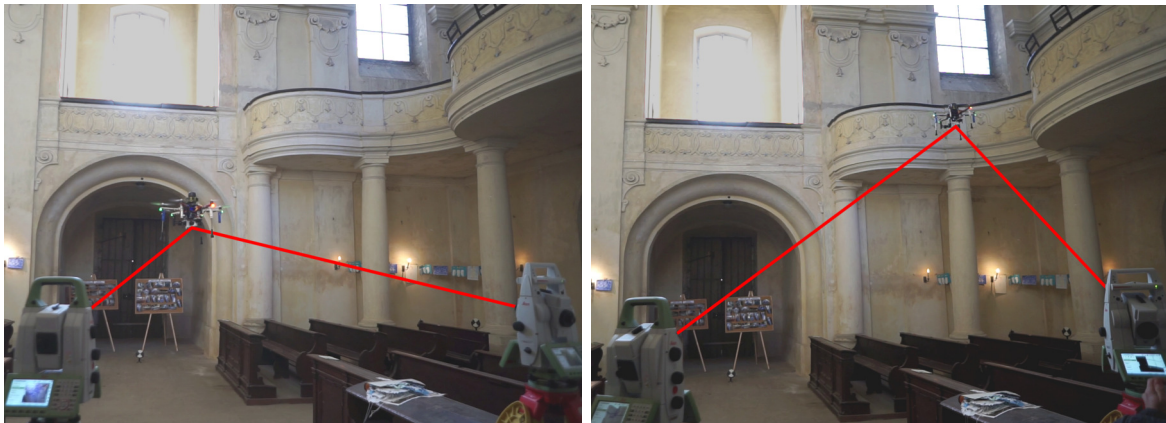
Figure 6.10: Demonstration of automatic tracking of a prism reflector mounted onboard a UAV by the Leica stations. The red lines are added to the picture to highlight the stations' laser beams measuring distance to the onboard reflector.
