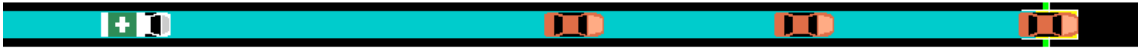
Figure 4.6: The resulting behaviour of the queue discharge based preference. The EV reaches the queue at the time when all vehicles are going at saturation speed.
