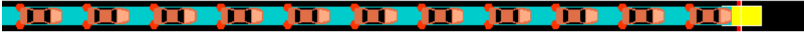
Figure 4.5: A queue of vehicles in SUMO . Yellow rectangle is E1 detector, light blue area is the E2 detector.
