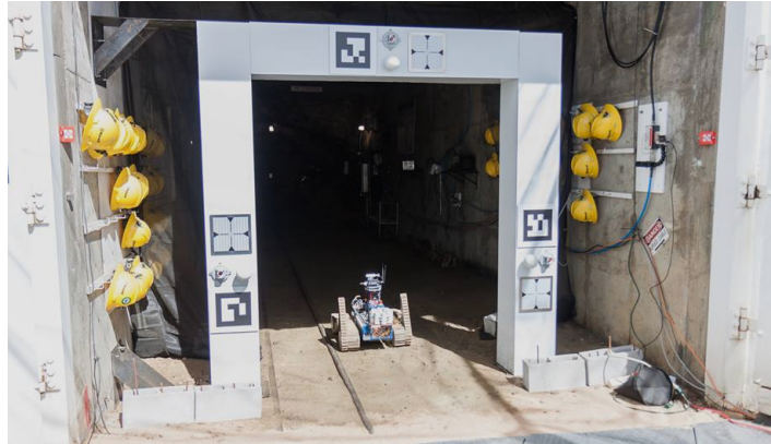
Figure 36: Tracked robot entering the experimental mine through the reference entry gate.
