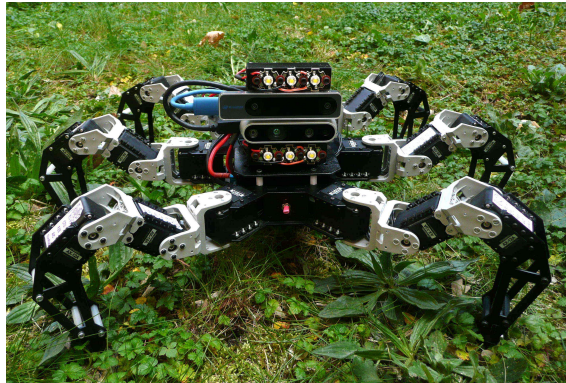
Figure 27: Hexapod walking robot with developed sensor rig designed for the exploration.
