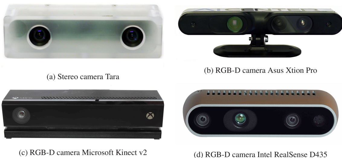
Figure 26: Sensors considered for vision-based localization.
