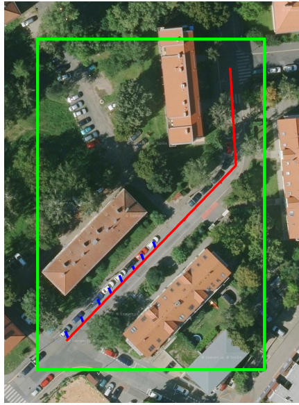
(a) Vršní, classified as one-side parking street with capacity 19 cars, real capacity \sim 16 cars.
