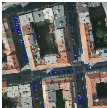
(b) Example of low accuracy of our detector over urban area with narrow streets and cars partially or fully in shadow.
