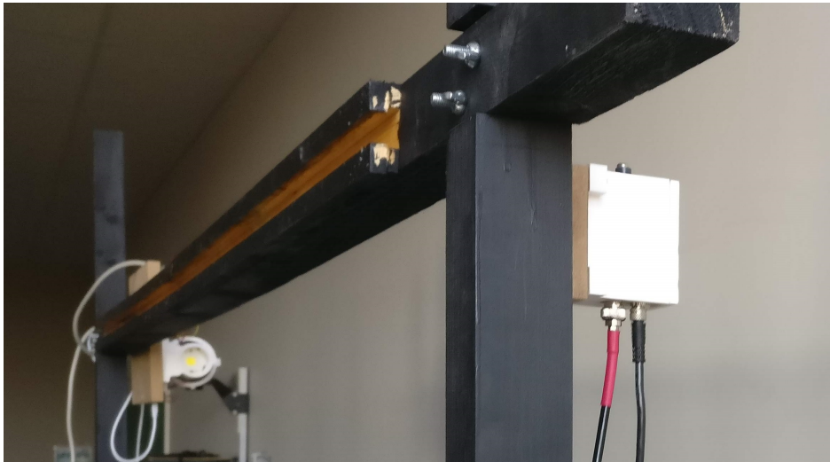
Figure 2.6: Photo of the whole setup with the TX part on the left and the RX part on the right.
