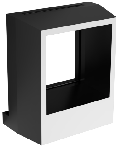
Figure B.2: 3D printable holder for polarizer, including collar guiding light from LED.
