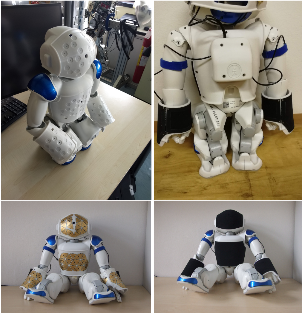
Figure 2.4: NAO robot with plastic mounts (top left), backpack for communications with the computer (top right), artificial skin (bottom left) and protective Lycra layers (bottom right).
