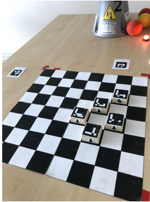
Figure 4.14: Experimental setup for robot accuracy test - moving knight piece between g6 and f4.
