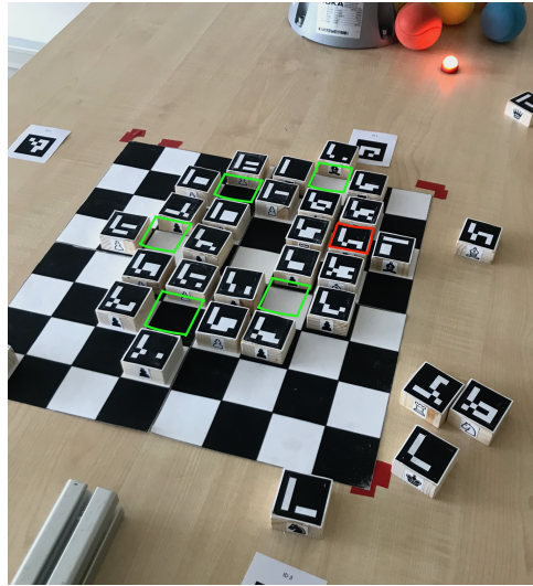
Figure 4.15: Experimental setup for robot accuracy test – moving knight piece around chessboard, knight initial position in red, way points in green.
