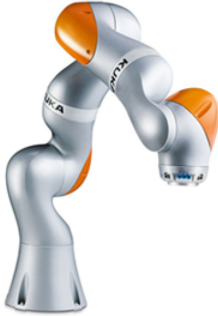
Figure 3.10: KUKA LBR Iiwa 7, from [kuk19].
