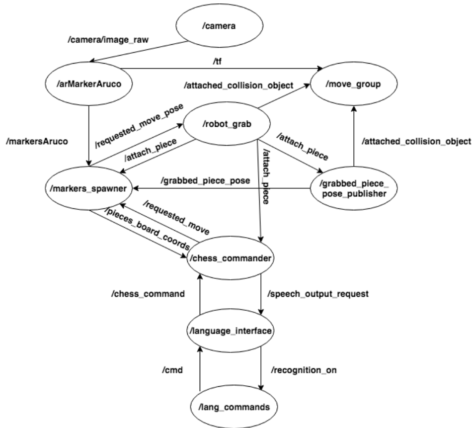
Figure 4.2: Project communication overview as rqt_graph , drawn using https://www.draw.io/ .
