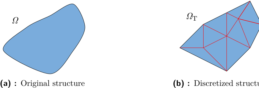
Figure 3.1: Illustration of discretization of a continuous shape (3.1a). Electromagnetic behaviour of a structure is approximated using its discretized model (3.1b).
