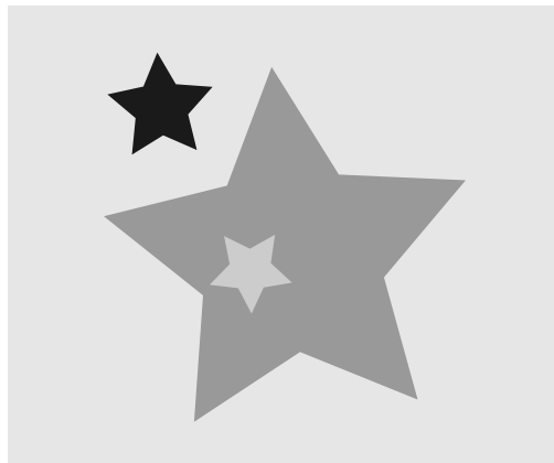
Figure 3.3: A sample image showing some of the redundancies which can be present in an image. As there are only 4 levels of gray color, storing them using 8 bits per possible gray color would result in high coding redundancy. Also, neighbouring pixels almost always have the same colors.
