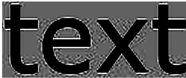
Figure 3.2: A zoomed in image used in the figure 3.1. While almost impossible to notice any artifact in the former example, the artifacts can be seen on the borders between the text and the gray background easily once zoomed in. Color levels were adjusted in order to emphasize the presence of artifacts.
