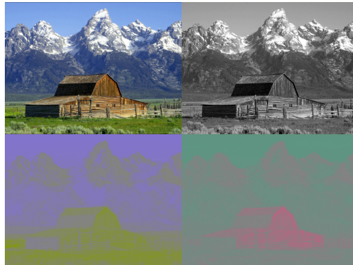
Figure 2.3: An image decomposed into the Y' , C_B and C_R components, as used in the Y' C_B C_R color space. The Y' component also represents the grayscale image.
