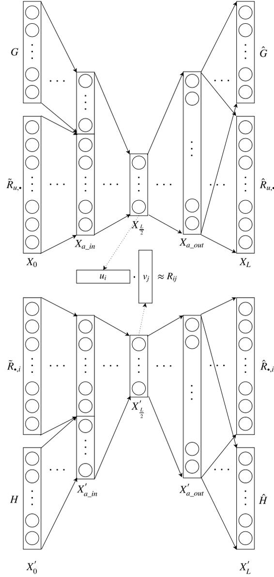
Figure 3.4: Hybrid Concatenated SDAE network architecture.
