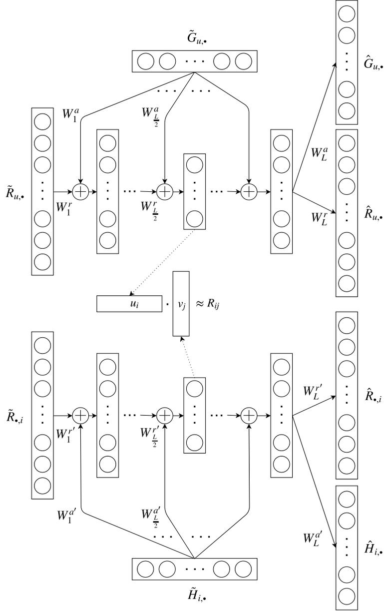
Figure 3.3: Hybrid Additional SDAE network architecture.
