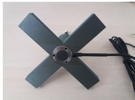
(b) Detail of the force sensor implemented into mechanism.
