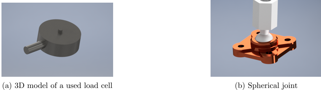
Figure 4.3: Components used in model. (a) shows the 3D model of the load cell and (b) shows flange bearing which is mounted on the plate.
