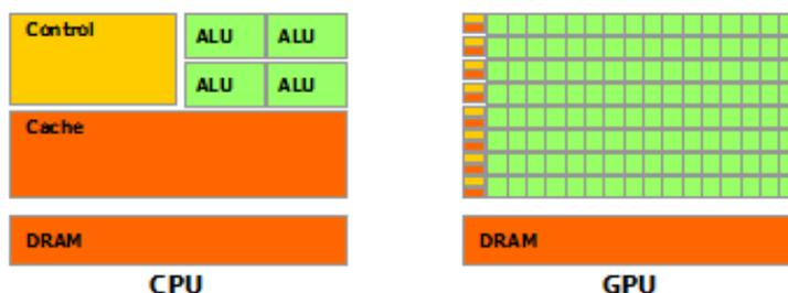
**Figure 3.1.** Simplified chip schematic of CPU (on left) and GPU (on right)[14]
