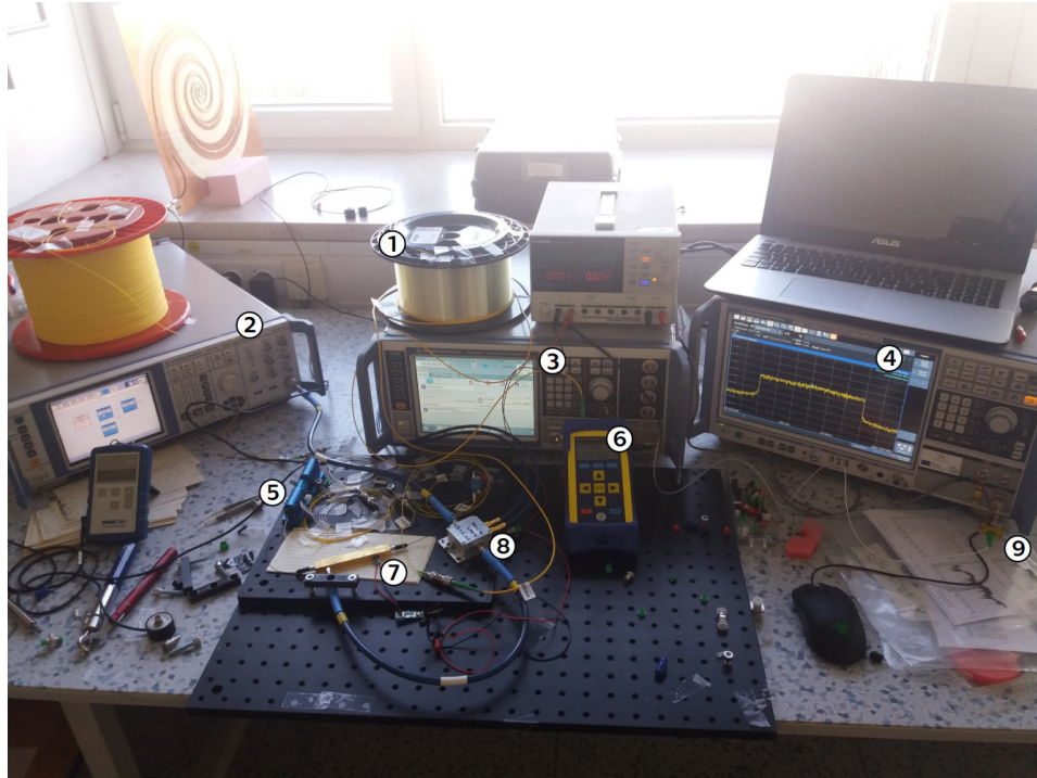
Figure 3.14: Laboratory RoF transmission link: 1 – 5 km fiber; 2 – SMF100A RF generator; 3 – SMW200A vector signal generator; 4 – FSW signal analyzer; 5 – Polarization controller; 6 – Variable optical attenuator; 7 – FTM7938EZ MZM; 8 – HMC 1041LC4 mixer; 9 – PD-40-C photodiode
