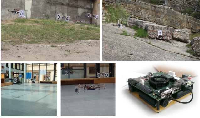
Fig. 2. Examples of the outdoor experiments of stabilization of MAV formations using the onboard vision-based relative localization system [1], [2] and picture of the 360° relative localization module.
