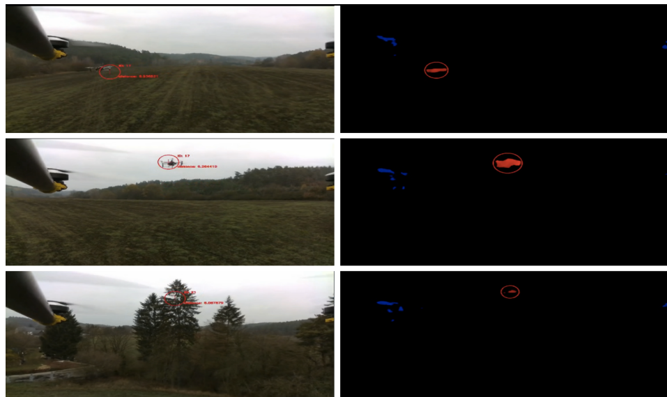
Figure 13: Examples of pictures obtained by onboard cameras for visual drone detection. Left: images taken by an RGB camera. Right: images taken by Intel RealSense Depth Camera. The red blobs represent the detected drone, while the blue blobs are caused by propellers and are not considered in the object detection algorithm.
