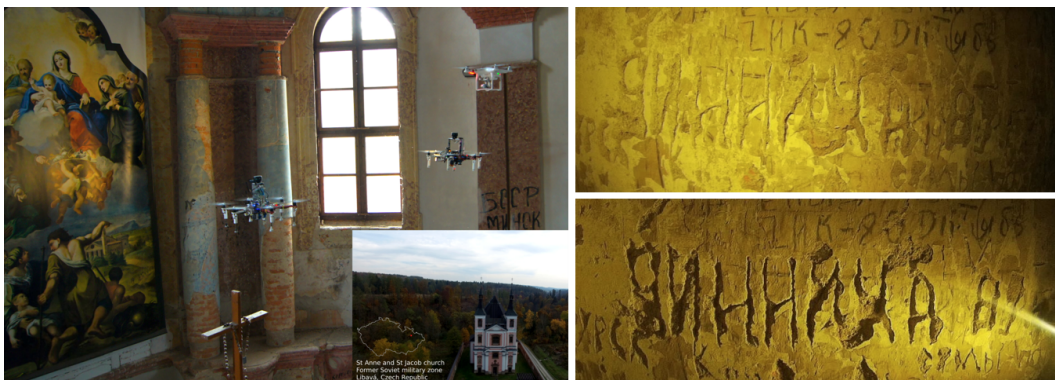
Figure 19: Documentation and exploration works in a church in Stará voda village, which was a part of the Libavá military region and training area. A formation of cooperating MAVs provided a set of pictures of difficult-to-access parts of the church and statues damaged by Czechoslovakian soldiers (before 1968) and by Soviet soldiers (after 1968). The upper right picture of the graffiti was captured by a single MAV carrying both the camera and the light, while the bottom picture was taken by a pair of MAVs, one with a camera and the other with an external light.
