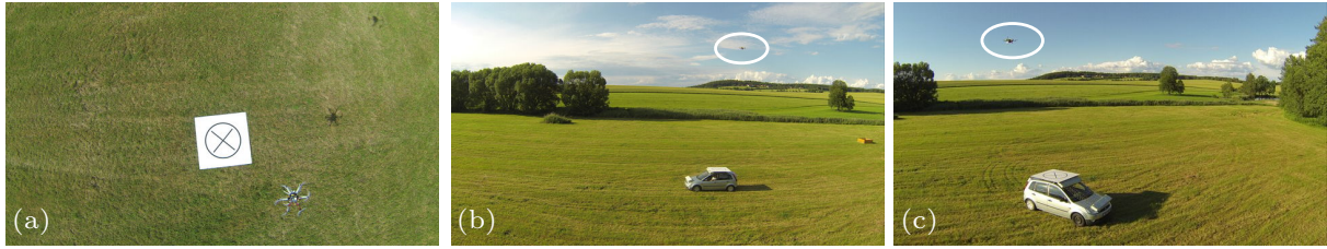
Figure 12: Photos from the first experiments in the field, a) shows a UAV hovering above a static target, b) shows a UAV tracking a vehicle moving along a linear trajectory, and c) depicts first attempts with tracking a ground vehicle moving in circles. The Linear Kalman Filter was used to estimate the states of the ground vehicle during this stage of development. Additional video material documenting these experiments can be found at http://mrs.felk.cvut.cz/jfr2018landing-video1 .
