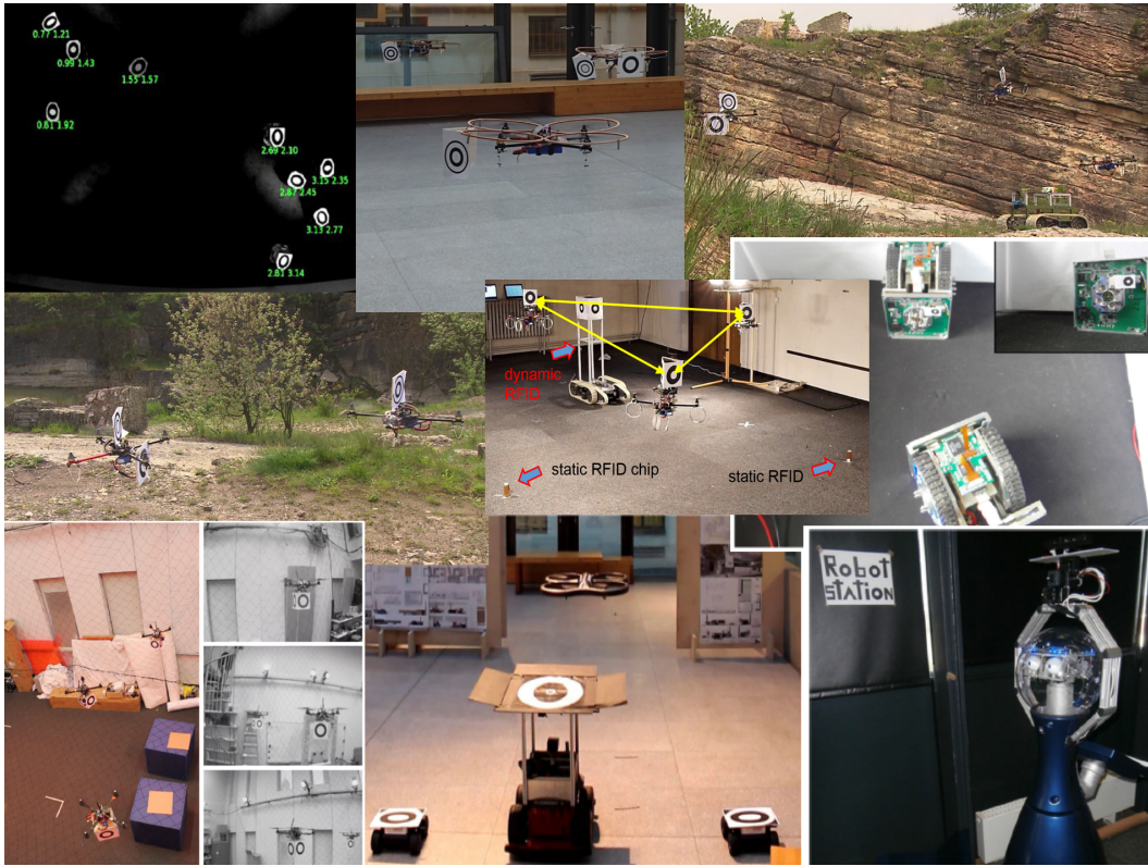
Figure 9: Examples of the deployment of the circle pattern detector published in [12] and [7]. This picture was composed with the help of Tomas Krajník, the main author of the circle detector [7], and other co-authors.
