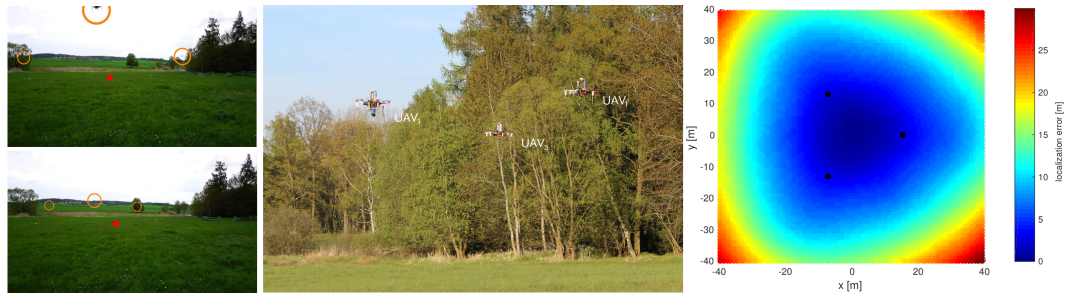
Figure 25: Snapshots from experiments with a formation of MAVs carrying directive (left) and rotating omnidirectional (middle) onboard antennas. The picture on the right side demonstrates the influence of the localization error on the shape and position of the formation. Source: [36].
