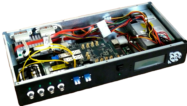
Figure 5.1: A physical view of the adapter that utilizes the embedded TIC.
