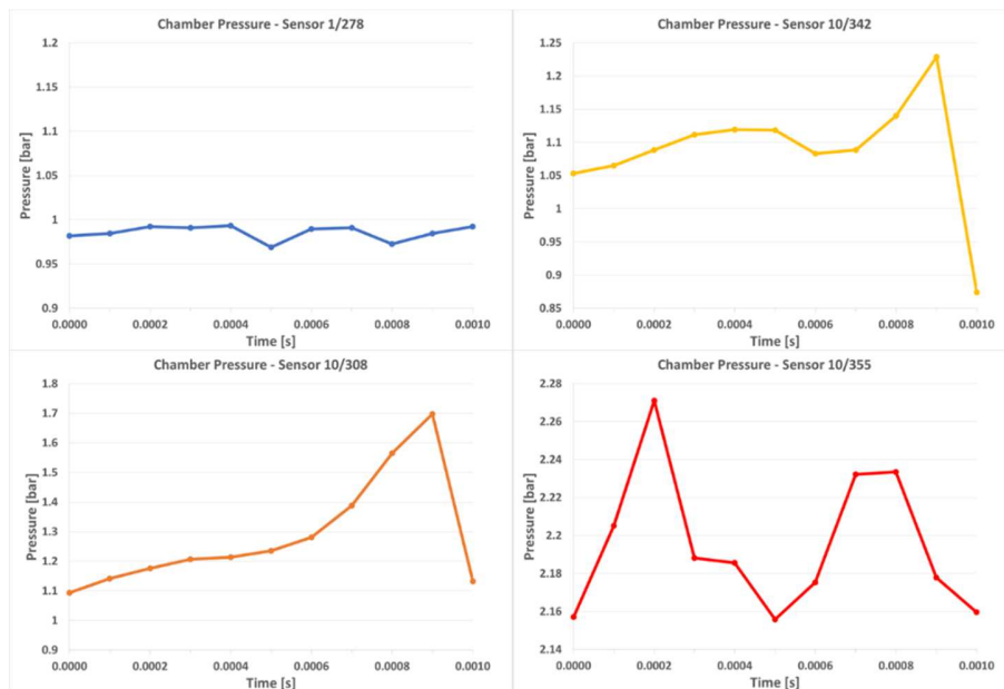
Figure 6-9: Pressure values from each sensor corresponding to one cycle (at time base at this stage) (R-type supercharger)
