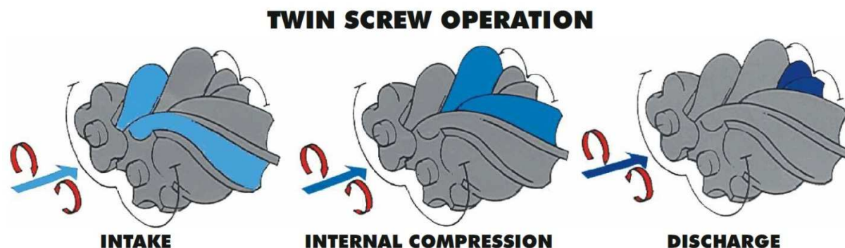
Figure 2-3: Screw compressor operation [9]
