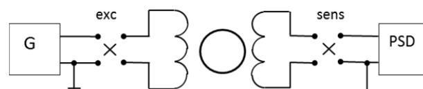
Fig. 1 Schematics of the fluxgate sensor excited by the generator G and at the output connected to lock-in amplifier (phase-sensitive detector PSD).
