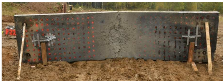
Fig. 1. Prepared specimen in vertical position with two explosive charges located in the centre of the both side parts.
