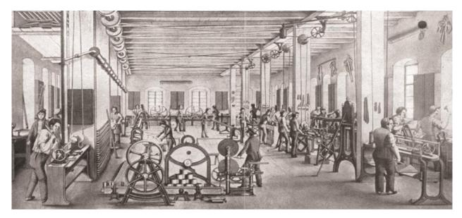
Fig. 1. Distribution of mechanical energy: manufacturing workshop of Bracegirdle machinery factory in Jablonec, 1840 [12]
