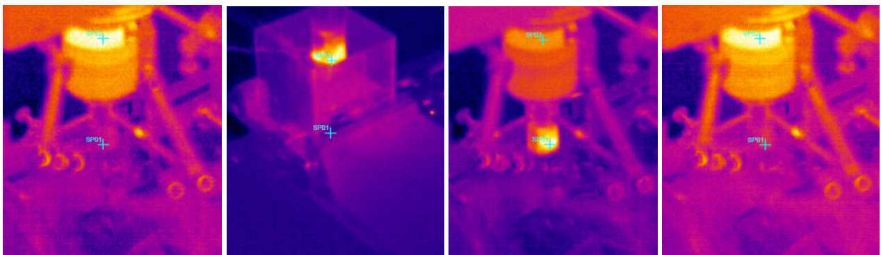
Fig. 11. Infrared images taken during 2nd machining cycle and following cooling
