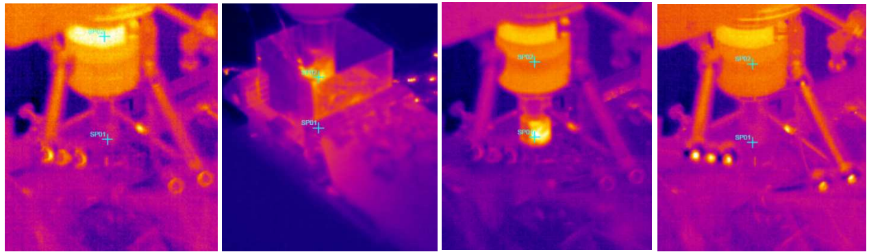
Fig. 13. Infrared images taken during 4th machining cycle and following cooling
