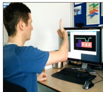
Fig. 7.4. Gesture control mapped to the incremental interface tested with the 3D tracking camera [16].
