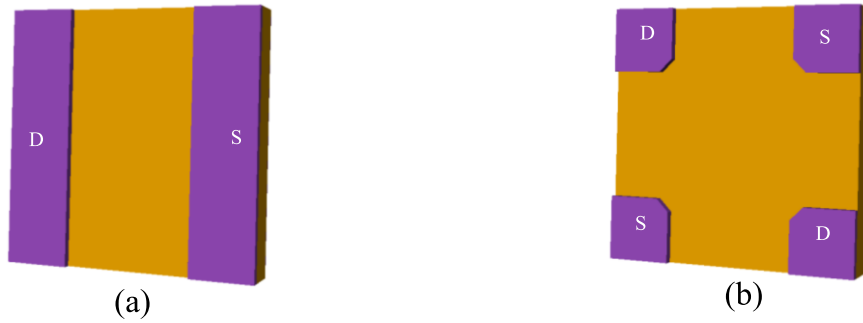
Fig. 5.5. Element for modeling Area Increment AI from R_{DS-ON} resistance for Normally-On Waffle GaN HEMT: (a) element of finger gate transistor, (b) element of new transistor with Waffle, where S is source and D is drain contact
