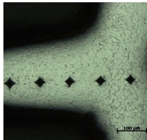
FIGURE 17. Half section of RBW 0.46 mm, etched Kroll.
