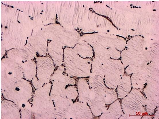
FIGURE 10. WM optical micrograph,  $\mu$ PAW, 5 A, 0.06 s, perfect Ar shielding, Kroll etchant, 280 HV, pink NiTi phase [12].
