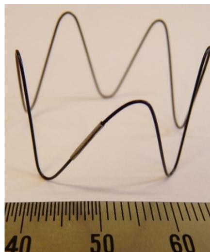
FIGURE 2. Crimped NiTi wire ( $\varnothing 0.45$  mm, shape set, dark oxide).
