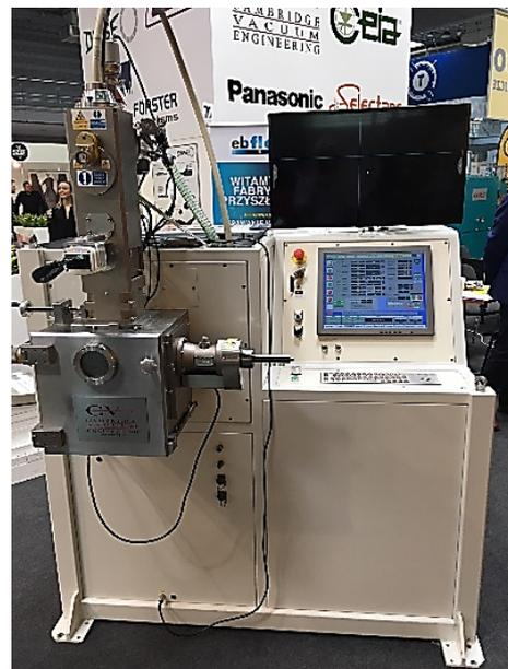
FIGURE 6. CVE – EBW welding source 60 kV.
