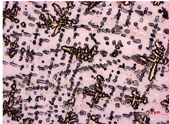
FIGURE 11. WM optical micrograph, imperfect Ar shielding  $\mu$ PAW, 5 A, 0.06 s, Kroll etchant, 550 HV, pink NiTi [12], precipitation of  $Ti_2Ni$ ,  $Ni_3Ti$ .
