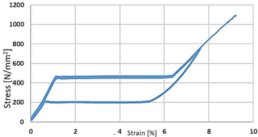
FIGURE 14. Stress-strain diagram of base material, tensile test, 4 cycles+till rupture.
