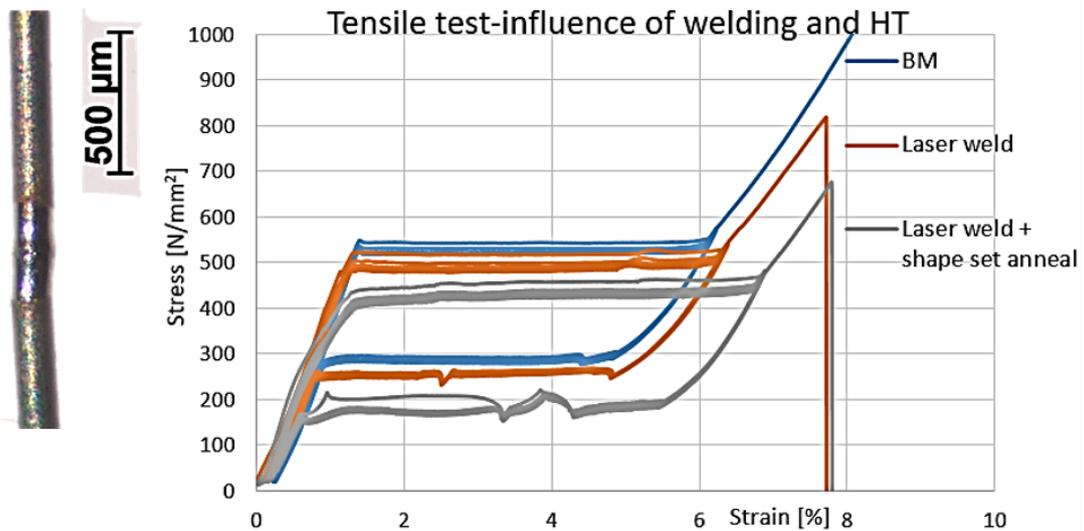
FIGURE 12. Tensile test,  $\varnothing 0.15$  mm (4 cycles + until rupture): (1) base material, (2) welded, (3) welded and shape annealed.
