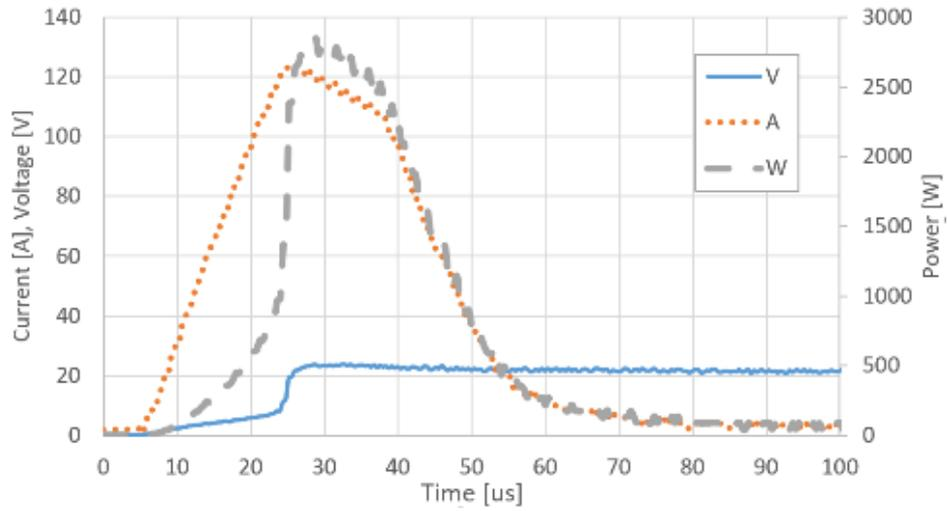
FIGURE 9. Capacitor pulse during the welding for used parameters –  $U$ ,  $I$ ,  $P$  in time.
