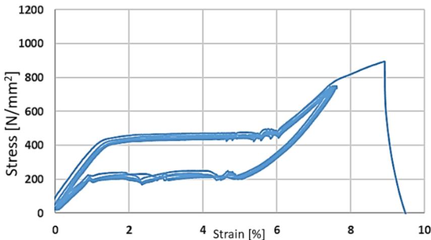
FIGURE 15. Stress-strain diagram of EWB sample, tensile test, 4 cycles+till rupture similar to BM, best result.
