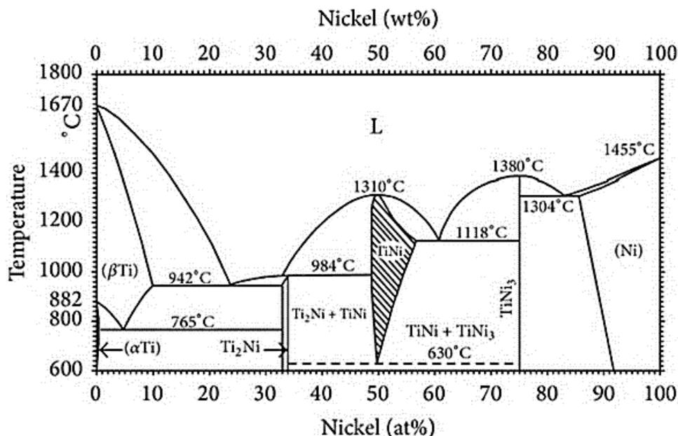
FIGURE 3. Binary diagram of Ni-Ti [2].
