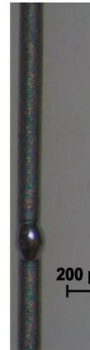
FIGURE 13. EBW weld, on 0.15 mm – 60 kV, 0.1 mA, pulse 10 ms, energy 0.1 J.
