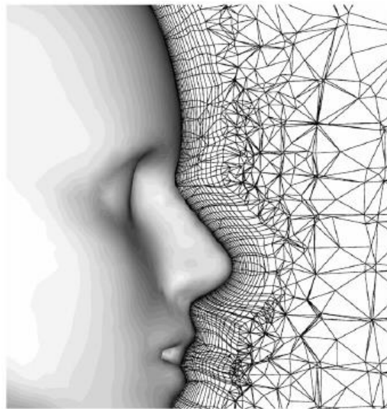
Fig. 2.11 – Numerical mesh near the face (Sørensen & Voigt 2003)
