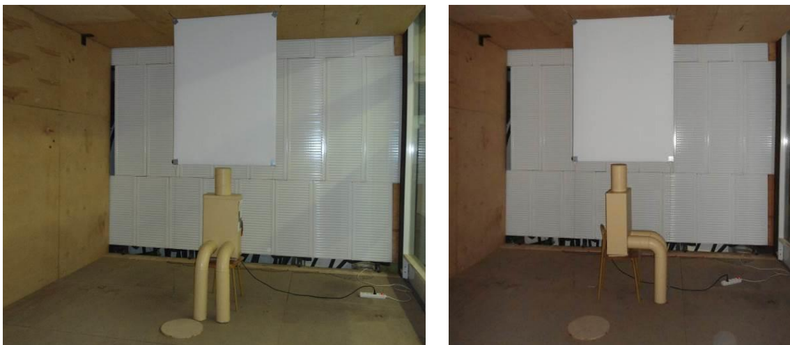
Fig. 4.3 – Experimental chamber with thermal manikin, 2 measured arrangements
