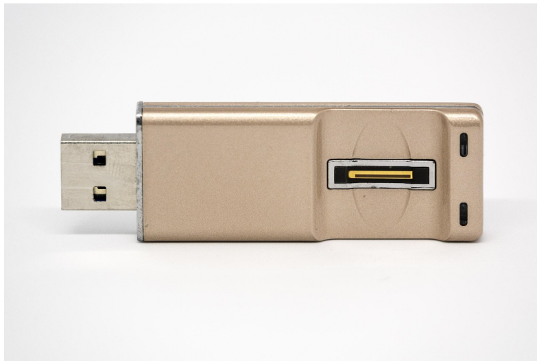
Figure 2.1: Generic flash drive with a fingerprint scanner[14]
