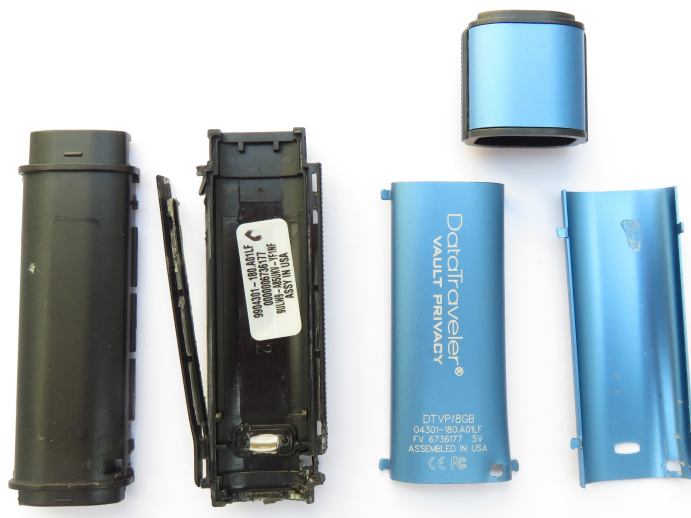
Figure 3.2: Enclosure taken apart
