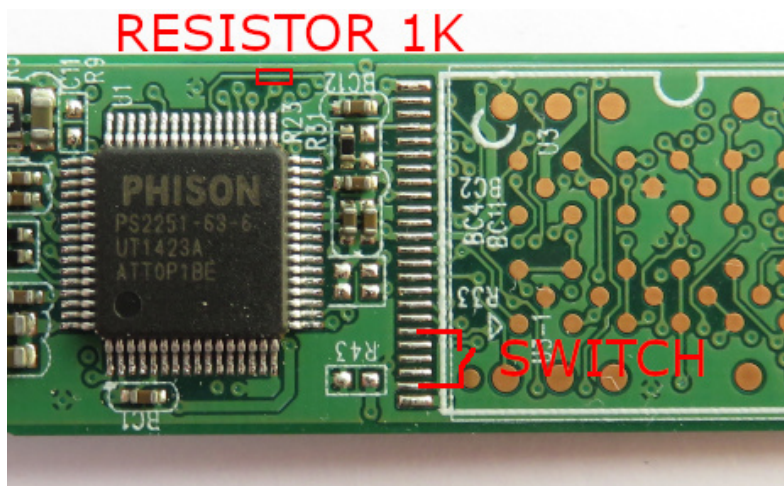
Figure 7.3: Safely tying the write protect pin to ground using a switch
