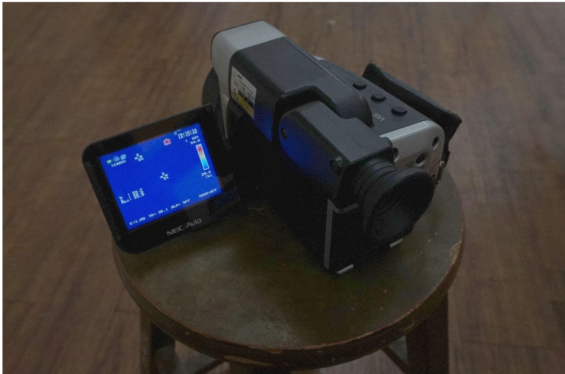
Pic. 16: Thermal-imaging camera InfReC R500EX Series '17/11
