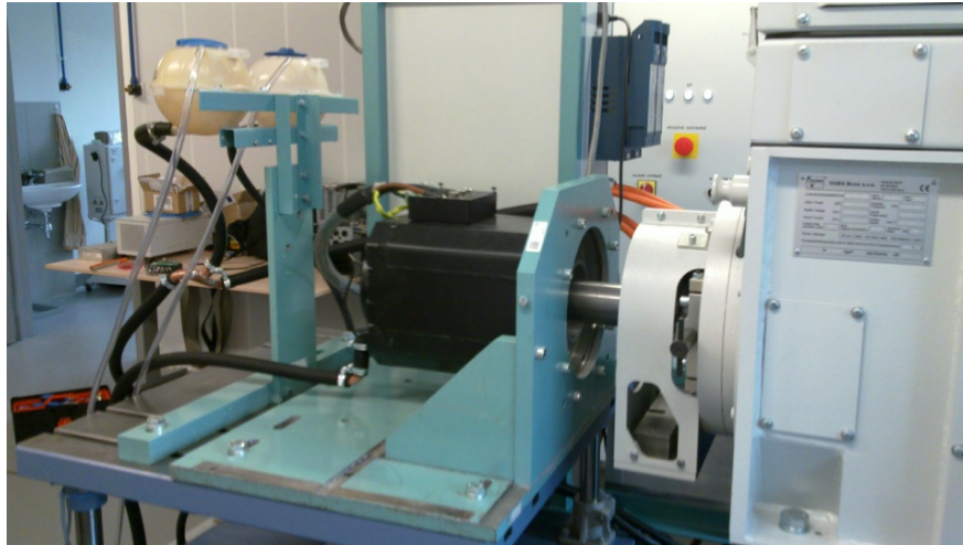
Tested Induction Motor connected to the Dynamometer
