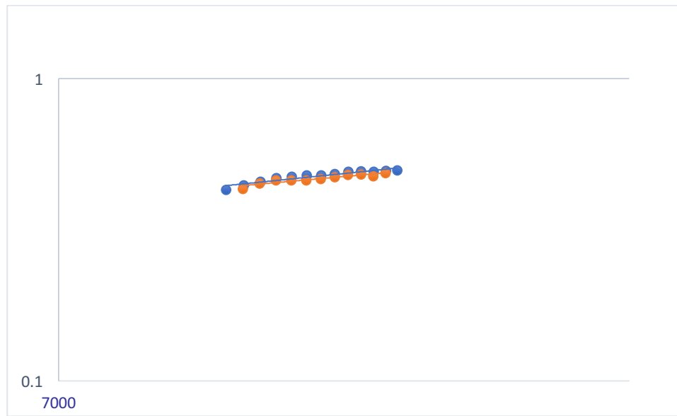
Figure 22. Variation of power number with Reynolds number for Impeller 4PBT in water ( Dv=70 , C=D_{imp} )
