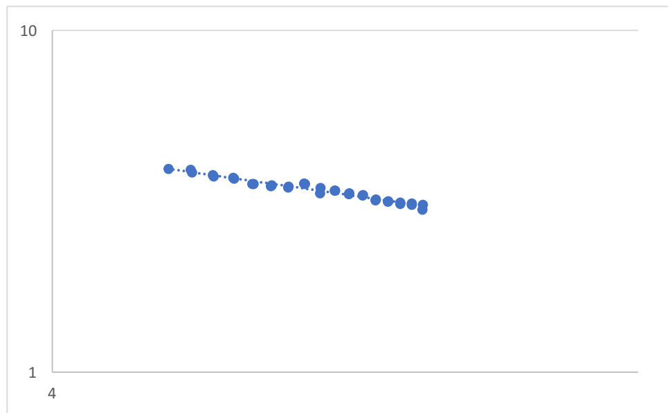
Figure 40. Variation of power number with Reynolds number for Impeller 4RT in Glycerine ( D_v=70 , C=0.5D_{imp} )
