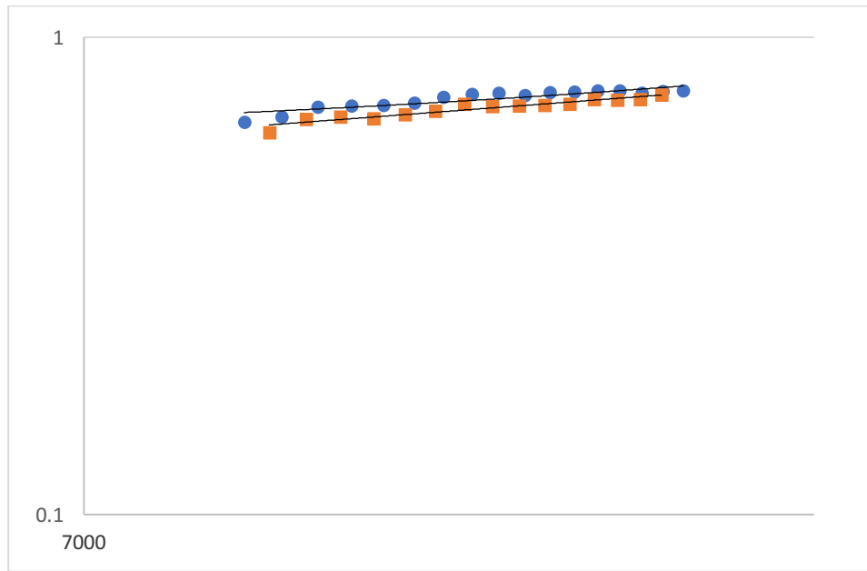
Figure 21. Variation of power number with Reynolds number for Impeller 4PBT in water ( Dv=70 , C=0.5D_{imp} )
