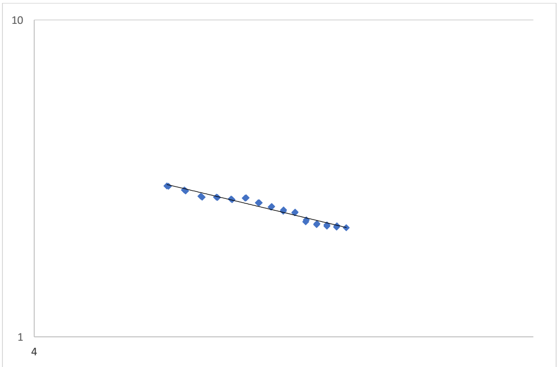
Figure 41. Variation of power number with Reynolds number for Impeller 4BTT in Glycerine ( Dv=70 , C=0.5D_{imp} )
