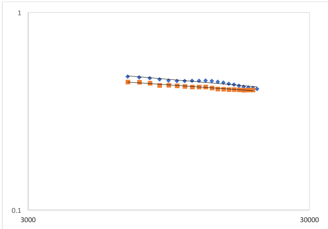
Figure 23. Variation of power number with Reynolds number for Impeller Anchor in water ( Dv=70 , C=0.055D_{imp} )
