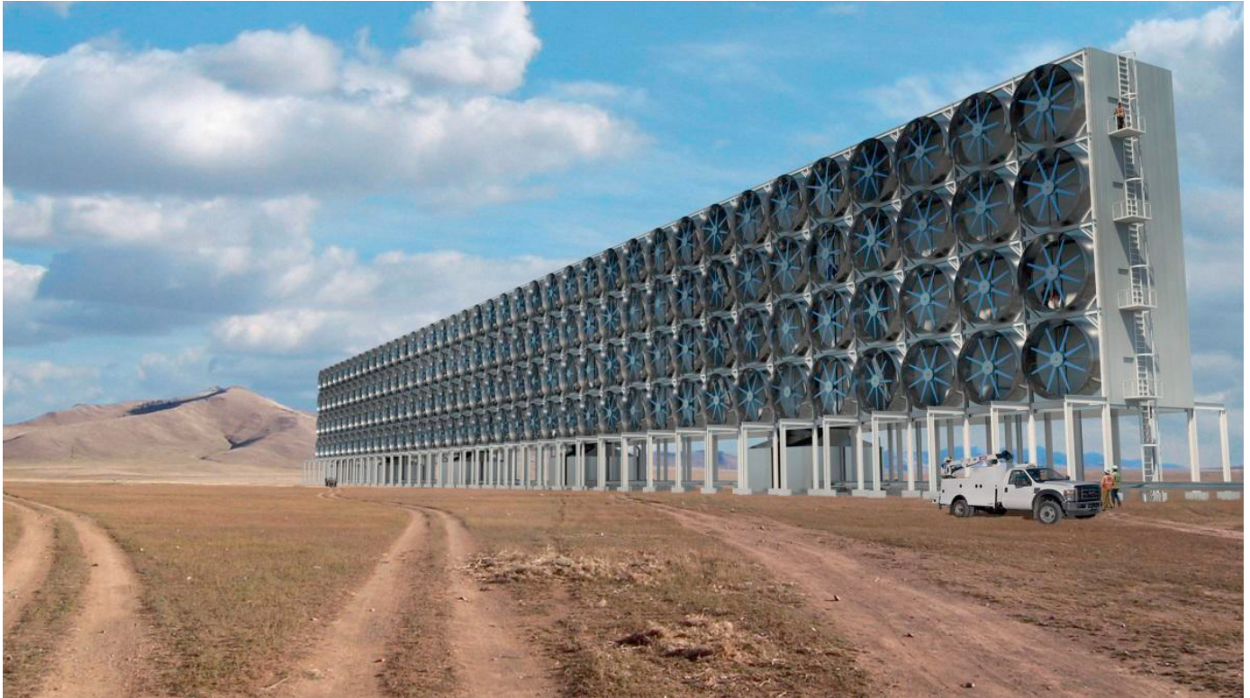
Figure 8: Rendering of CE full-scale slab contactor design. This module would capture 100 kt-CO 2 /yr. (source: Outdoor prototype results for direct atmospheric capture of carbon dioxide , GeoffreyHolmes )
