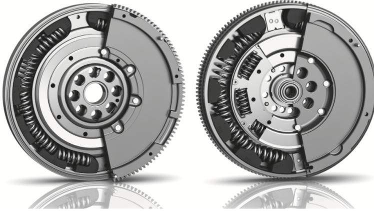
*Figure 2.3.4- DMF with straight pressure springs on the outer (both) and inner radius (inner damper-right)*
